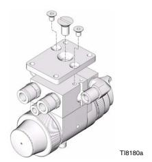
Fig. 7: Retrofit Adapter Plate Mount
